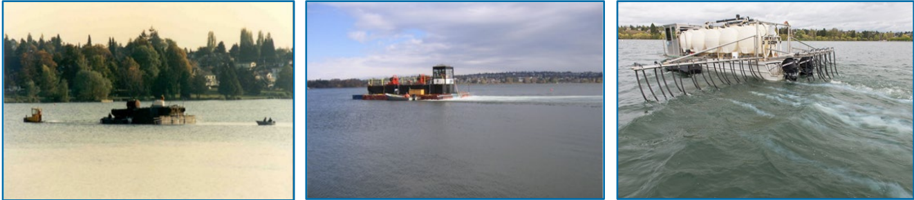
Figure 7. Buffered Alum Treatments in 1991, 2004, and 2016 (left to right) for Sediment Phosphorus Inactivation in Green Lake, Seattle.
